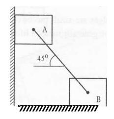
Since the bar is in compression, the compressive force is directed towards the ends of the bar as shown in the free - body diagram of blocks A and B
