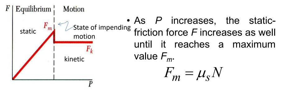
• Further increase in P causes the block to begin to move as F drops to a smaller kinetic-friction force  $F_k$ .
