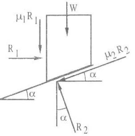
Find the horizontal force P on the 10° wedge shown in fig. to raise the 1500 N load. The coefficient of friction is 0.3 at all contact surfaces
