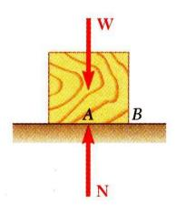
• Block of weight *W* placed on horizontal surface. Forces acting on block are its weight and reaction of surface *N*.
