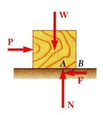
• Small horizontal force *P* applied to block. For block to remain stationary, in equilibrium, a horizontal component *F* of the surface reaction is required. *F* is a *static-friction force*.
