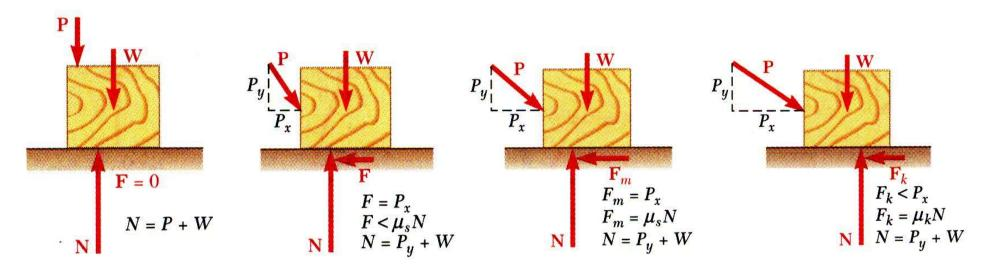
• No friction,  $(P_x = 0)$ • No motion,  $(P_x < F_m)$ • Motion impending,  $(P_x = F_m)$ • Motion,  $(P_x > F_m)$  • Consider block of weight W resting on board with variable inclination angle  $\theta$ .
